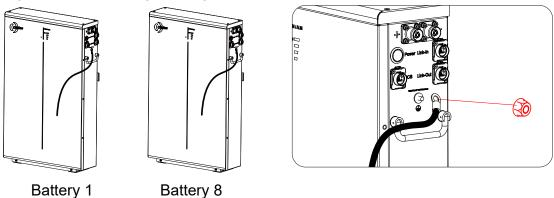
Step 3. Insert network cables into battery terminals.
