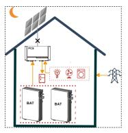
Battery powers loads at nighttime when there is no PV. If battery energy is insufficient, it can power loads together with grid.
