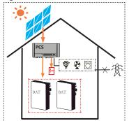
When grid falls, battery and PV can power loads.
