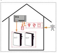
Battery can be charged by grid. Users are suggested to store energy from grid to battery when electricity price is relatively lower.
