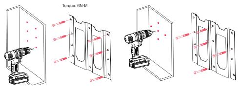
Step 3. Fix battery on bracket.
