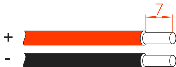
Figure3-38 Stripping diagram of DC input (unit: mm)
