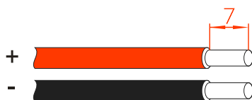
Figure 3-32 Stripping diagram of DC input (unit: mm)
